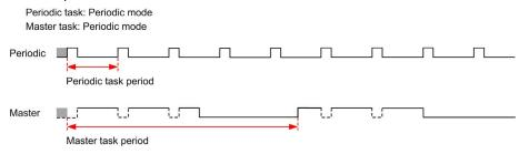
If the processor goes to the HALTED state when the master task is configured in freewheeling mode, verify whether the periodic task scan delay time is significant in comparison to the periodic task period. If so, try:
